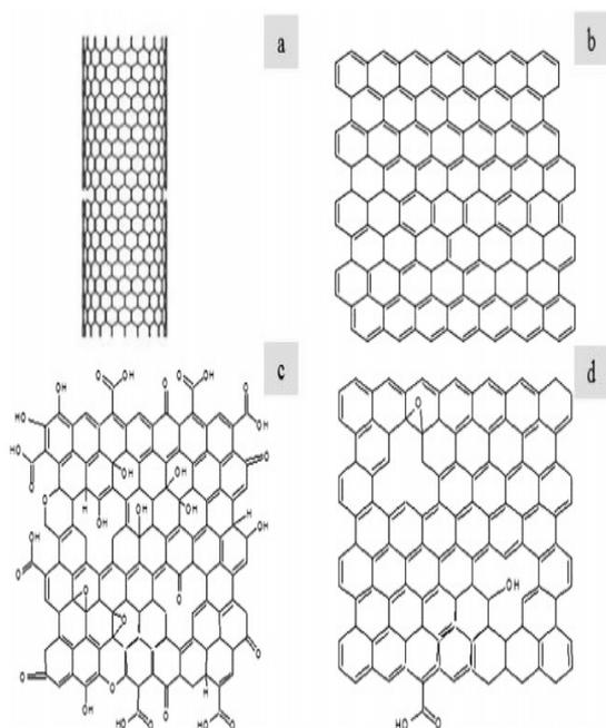
**Fig. 2.4.** Displays the structure of different forms of carbon (a) Carbon Nanotube (b) Graphene (c) Graphene Oxide (d) Reduced Graphene Oxide.
