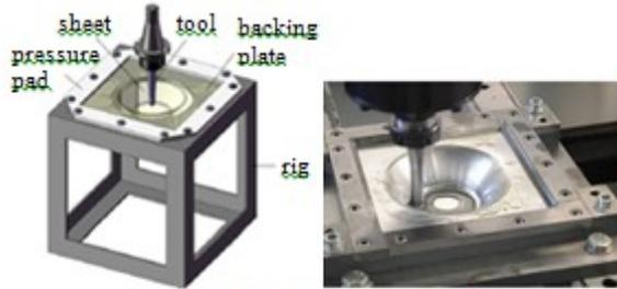
Fig. 2.1 Clamping system for SPIF
