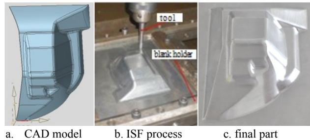
Fig. 4.1. Automotive body panel manufactured by ISF. Source: [36]
