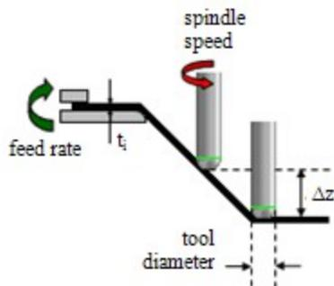
Fig. 3.3 The main process parameters
