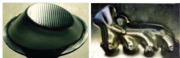
Fig. 4.4. Automotive components made by ISF
