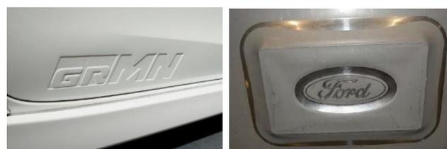
Fig. 4.3. Logo mark made by ISF on existing components
