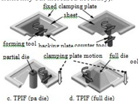
Fig.1.1 Incremental forming configurations. Source: [2]
