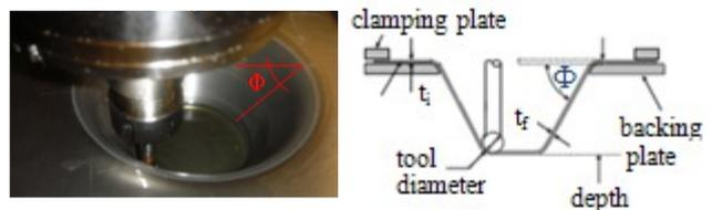
Fig. 3.2. The maximum forming angle
