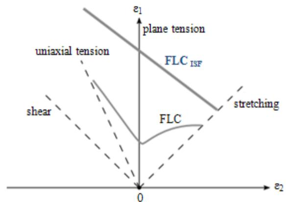
Fig. 3.1. Forming limits in conventional forming versus incremental forming
