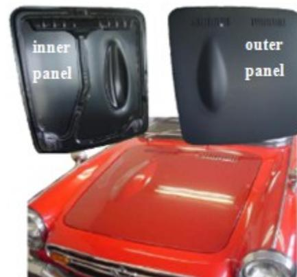
Fig. 4.2. Replacement Honda S 800 hood made by stretch forming and ISF. Source: [35]
