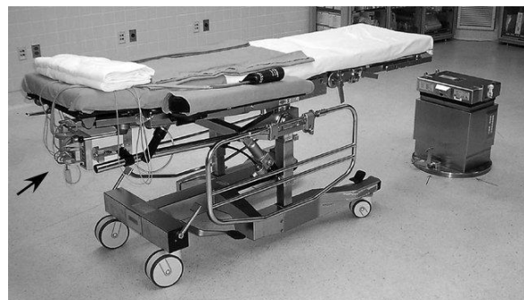
Fig. 2. Mobile operating tabletop, transporter, and fixed base column used to facilitate rapid movement of anesthetized patients between areas in the Operating Room of the Future[7]. Moreover, the Pediatric Physiotherapy Department’s devices should operate properly at indoors and outdoors in emergencies and should have good operation with other hospital units [13, 19, 20]. Hence, children that have been injured by several accidents could be recovered in time using proper supported electronic facilities.
